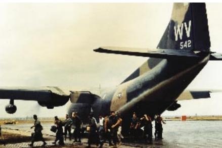
It was in this C-123K Provider that Jackson and his crew made their courageous rescue. The K model had small jet engines to assist in max-performance takeoffs. Ignoring safety, Jackson kept them at high power, keeping time on the ground to fewer than 50 seconds. Miraculously, not a single bullet hit the aircraft.
